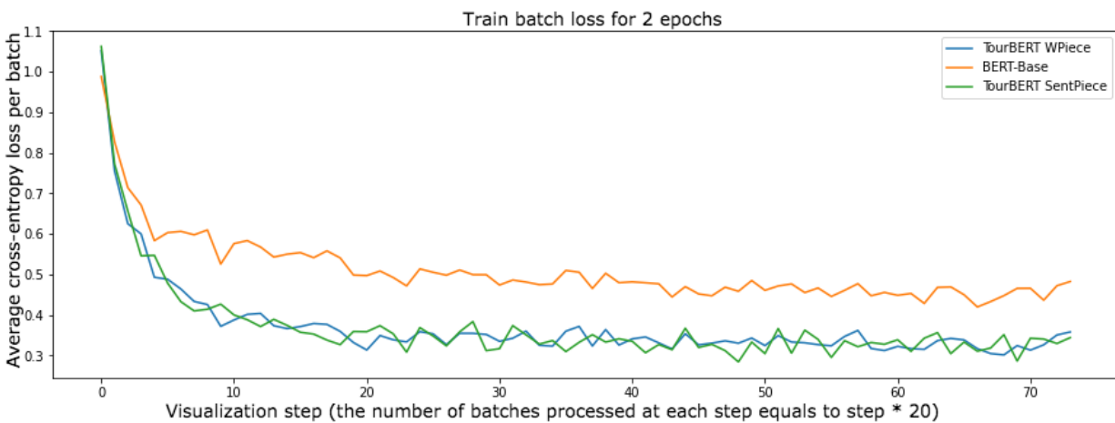
Figure 21: Batch cross-entropy loss of TourBERT and BERT-Base on training data for the multi-label classification task.
